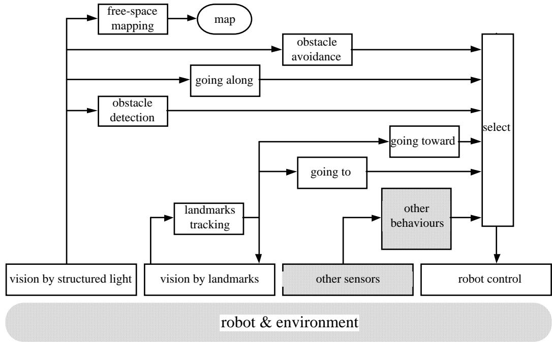
Fig. 2 Vision-based behaviours
