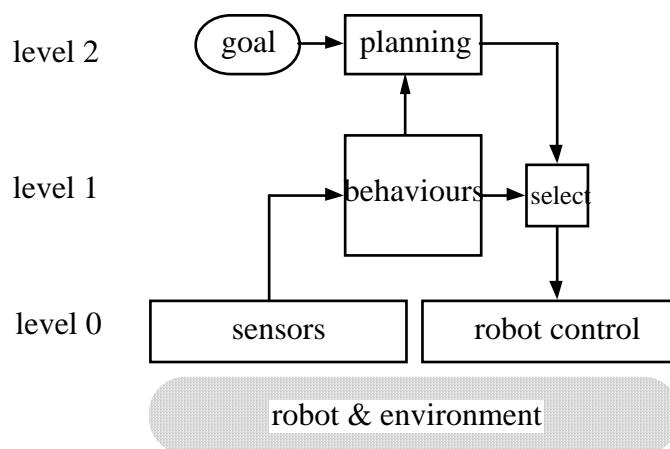
Fig. 1 Principle of the behavioural mobile robot navigation system
