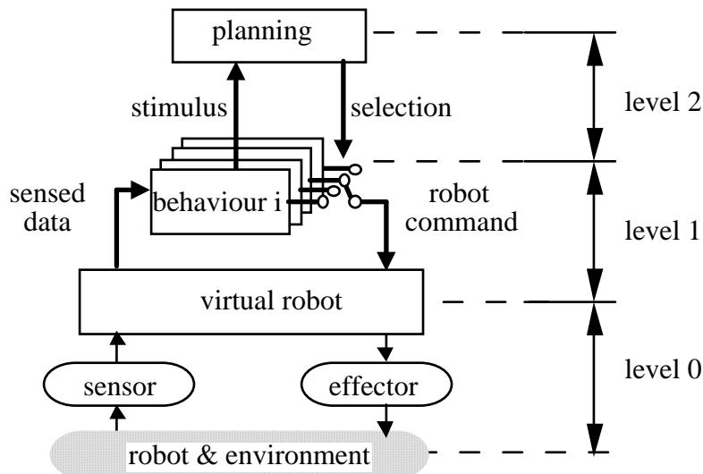
Fig. 4 Control structure of MANO
