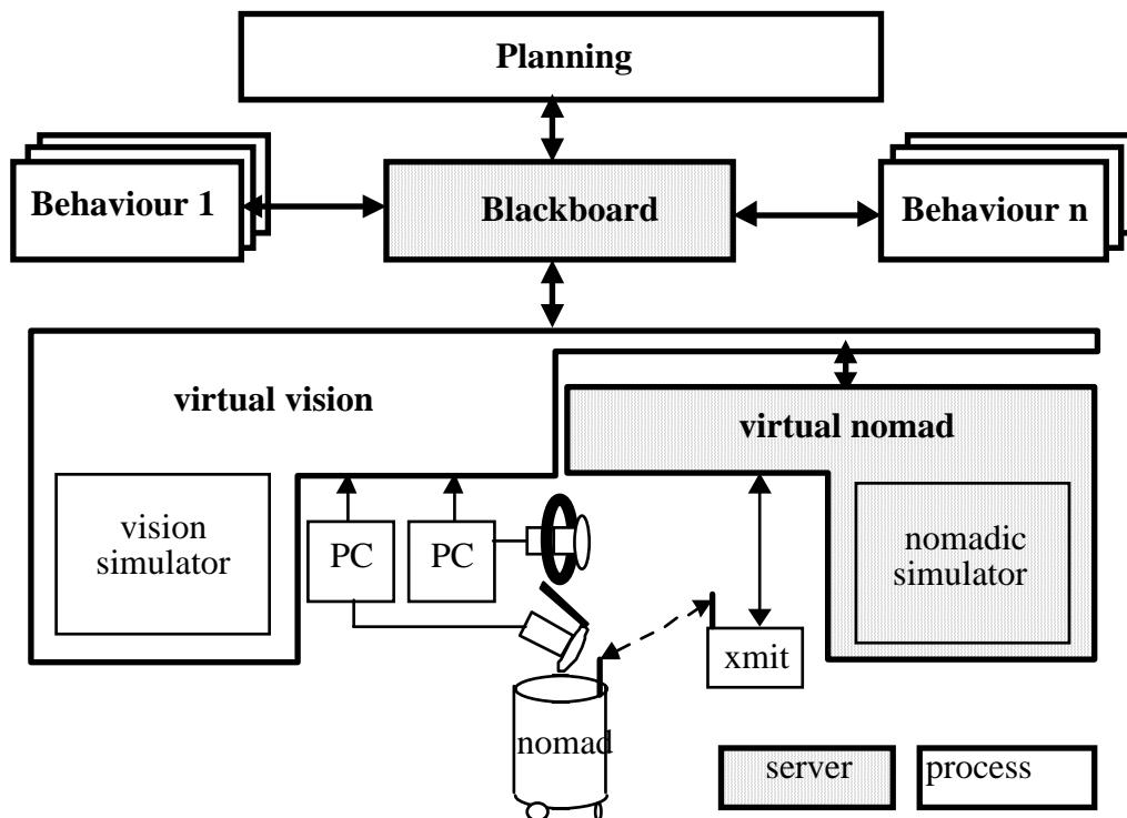
Fig. 7 Architecture and unix processes
