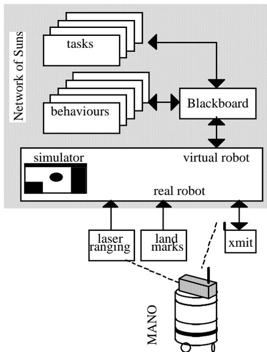
Figure 6: Experimental behavioural architecture
