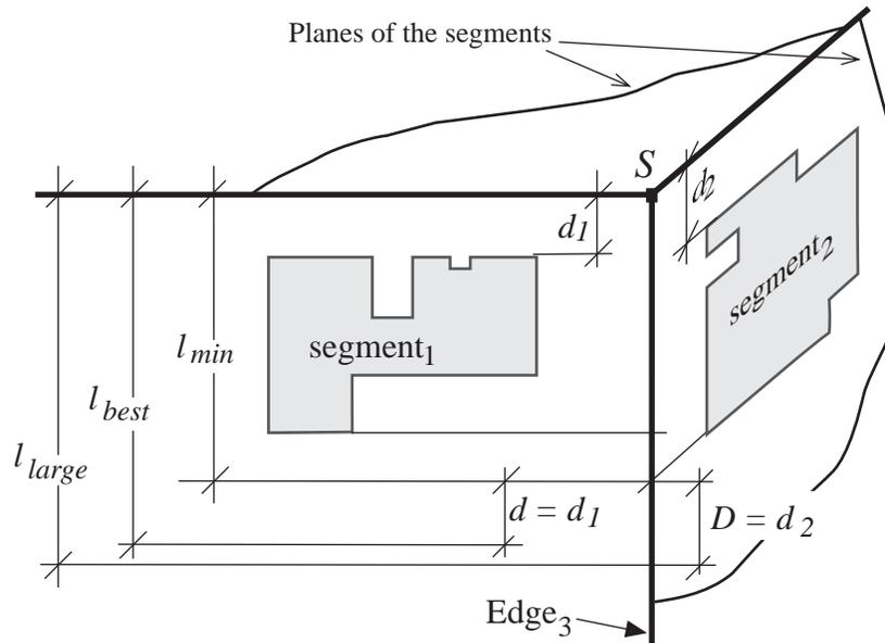
Fig. 3: Estimation of the length of one edge of the box
