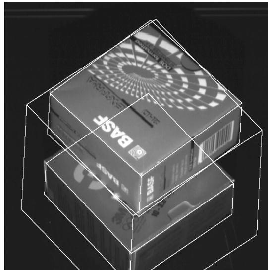
*Fig. 10: Intensity image with wire frames of box hypotheses. A false hypothesis is made due to a wrong grouping.*
