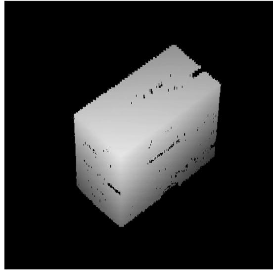
*Fig. 4 and 5: intensity and range image of a floppy box.*
