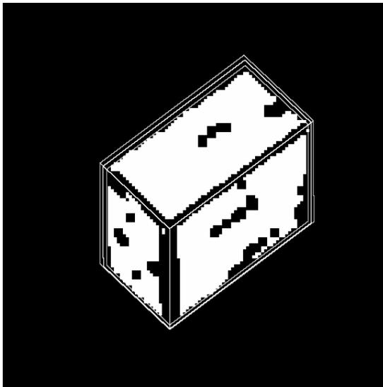
*Fig. 6: Result of segmentation, together with the wire frame of shape hypothesis. The three frames correspond to the three different size estimations.*
