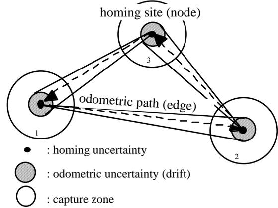
Figure 6: A triangle race navigation using visual homing sites and odometric paths between them
