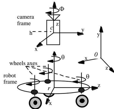
Figure 2: Nomad robot geometry with a vertical-mounted camera
