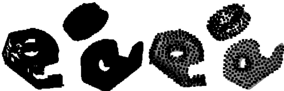
Fig. 5. Thresholded z-image and recognized models superposed to the intensity image
