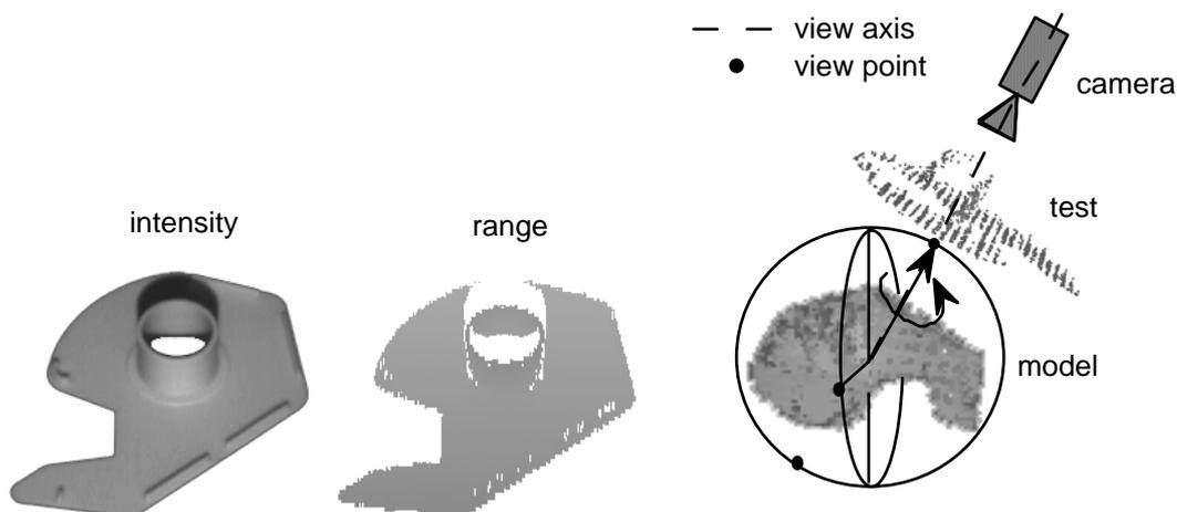
Fig. 2. Selection of starting configurations for a tape dispenser part
