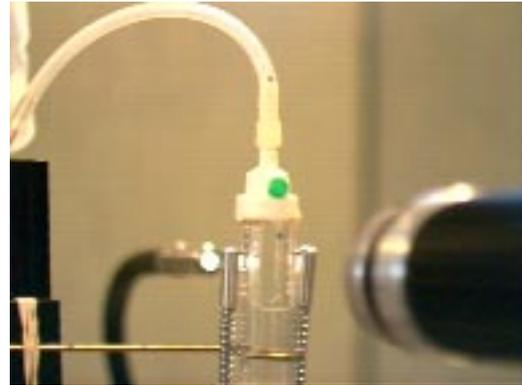
Fig. 3: Drop chamber and imaging section
